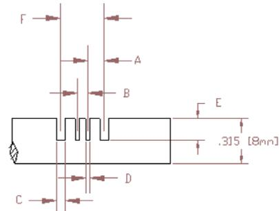
Wafer Slot Arrangement and Dimensions: Contiguous Carrier
